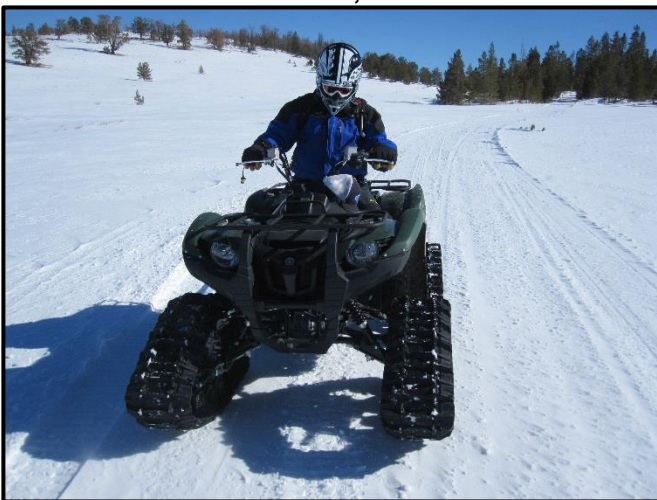
Photo 2-1: Tracked 2014 Yamaha Grizzly 700 46.5” wheeled width; 54” tracked width
