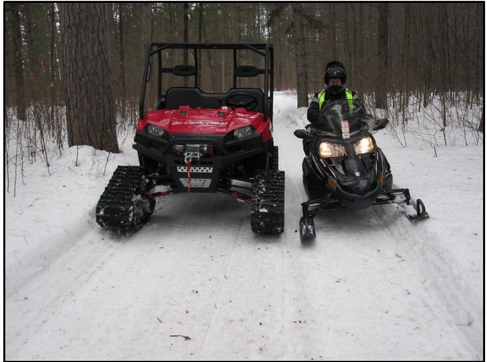
Photo 2-5: A tracked UTV beside a snowmobile on an 8'-6" (102") wide groomed snowmobile trail
