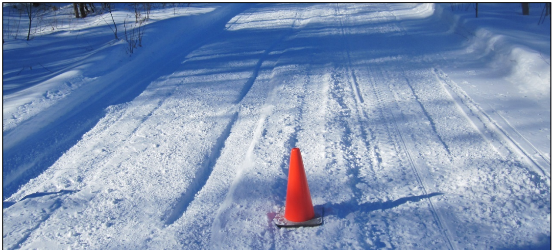
Photo 14: impressions from aggressive starts – (left side of photo) UTV #2 / RZR 1000 and (right side of photo) snowmobile #2 / RMK 600
